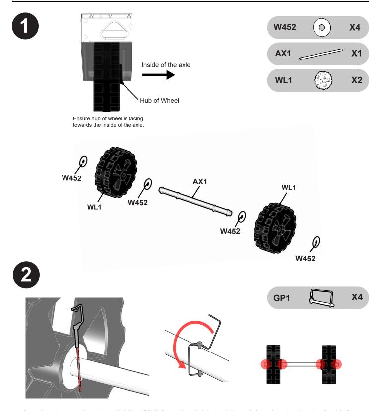
Open the retaining wire on the Hitch Pin (GP1). Place the pin into the hole and close the retaining wire. Do this for both sides of the wheel. Follow Step 2 for both ends of the axle.
