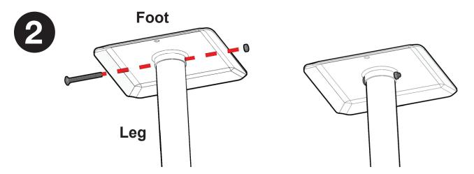
Unscrew the carriage bolts connected to the feet from the four legs that you removed from **STEP 1**. The legs will be used in assembling the axle in **STEP 3**.
