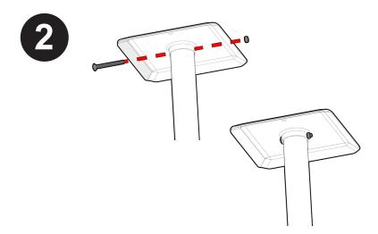
Unscrew any carriage Bolts connected to the feet (see above image). The legs will be used in assembling the axle in step 3.
