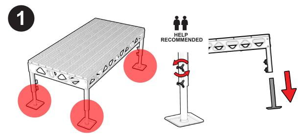
Loosen the adjustment clamps on each of the dock legs by turning the clamp knobs counter-clockwise (see image above). This will free the legs so they may be taken off the dock. It is recommended to use one person to hold a corner of the dock upwards while another person slides one leg off the dock at a time. Do this for any legs which will be used in the installation of the axle assembly.
