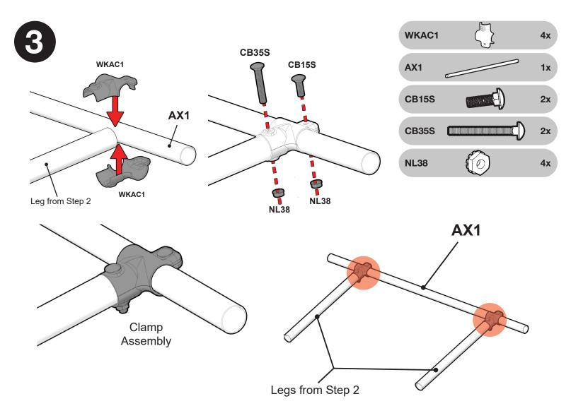
Install a clamp assembly for each side of the axle (AX1).
