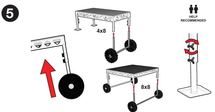
Use one person to hold a corner of the dock upwards. Insert one end of the axle assembly at a time into the legs of the dock. \*If there is more than one wheel kit to install then repeat **STEPS 1-5** for the other legs of the dock. Adjust the legs appropriately to the depth of water that you will be installing the dock in. Tighten the adjustment knobs to secure the height of the legs.
