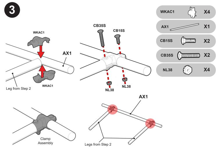
Install a clamp assembly for each side of the axle (AX1).
