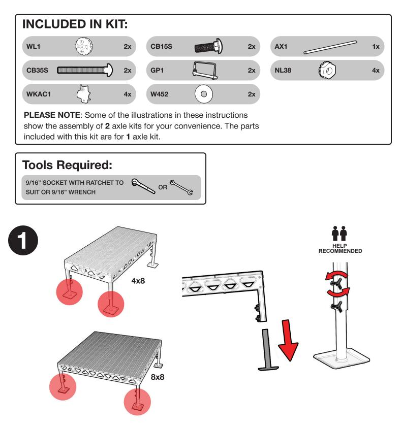
Loosen the adjustment knobs on each of the dock legs by turning the knobs counter-clockwise (**see above image**). This will free the legs so that they can be taken off the dock. It is recommended to use one person to hold a corner of the dock upwards while another person removed the legs, one at a time.
