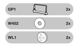
Slide the wheel (WL1) and washer (W452) onto the assembled frame (see above image). Slide open the retaining wire on the hitch pin (GP1). Place the pin into the holes on either side of the axle (AX1). Close the retaining wire on the hitch pin (GP1). Repeat this step for all axle ends.
