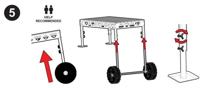
Use one person to hold a corner of the dock upwards. Insert one end of the axle assembly at a time into the legs of the dock.\* Perform this step for both axle assemblies. If there is more than one axle to install repeat this step for the opposite end of the dock in. Adjust the legs appropriate to the depth of water you will be installing the dock in. Turn the adjustment clamps clockwise to tighten the legs to your desired height.
