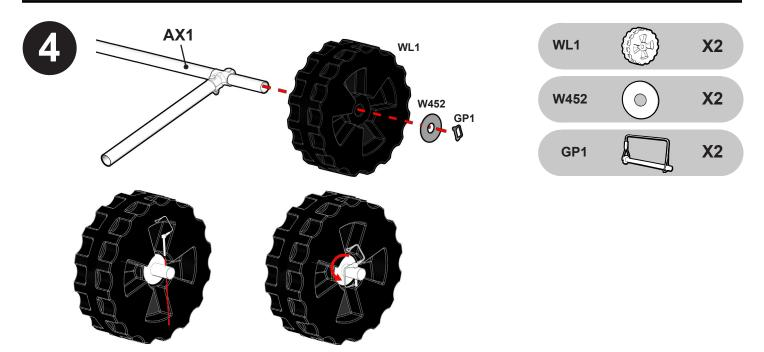
Slide the Wheel(WL1) and Washer (W452) onto the assembled frame (See above). Slide open the retaining wire on the Hitch Pin (GP1). Place the pin into the holes on either side of the Axle (AX1) (See above). Close the retaining wire on the Hitch Pin (GP1). Repeat this step for all axle ends.
