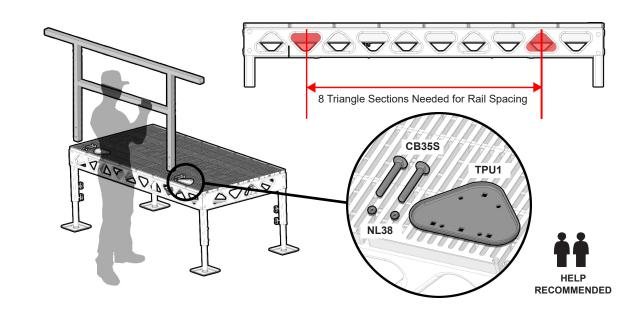
Find an area on your dock that will have 8 triangle sections between the railing. Organize and set all the hardware you will need (**Items TPU1, CB35S, NL38**) onto the decking near each point of fastening. Using the help of another person, hold the end of the railing level near the triangle cutout where it will be installed.
