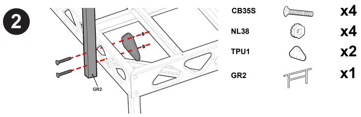
With one person holding the railing level place the **Triangle Backing Place(TPU1)** on the inside of the truss triangle cutout and fasten. Do this for both ends of the Hand Railing frame.
