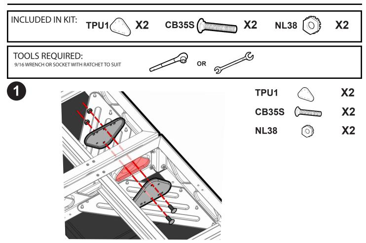
Triangle plates used for coupling docks can be attached using Carriage Bolts (CB35S) and Locknuts(NL38) (as shown above).
