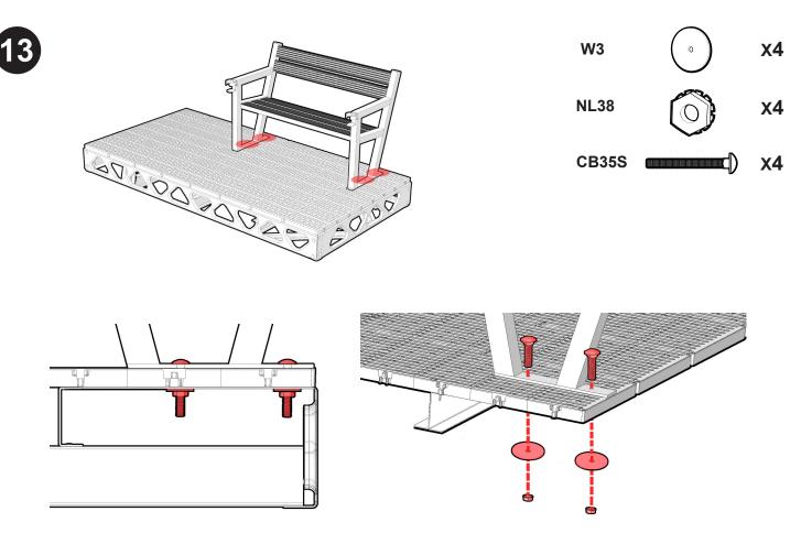
Connect carriage bolts(SB35S) with washers(W3) and lock nuts(NL38) as shown for both sides of bench.
