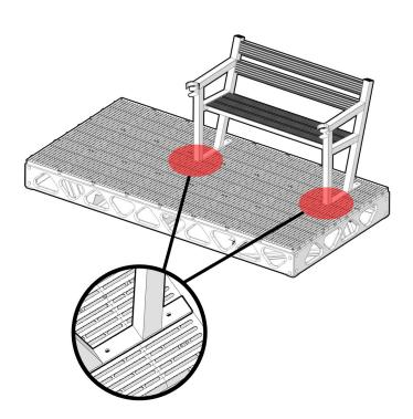
Line up bench bracket holes with slots in decking.
