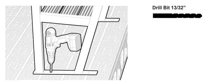
**TIP:** Sometimes the holes in the decking do not line up with the bench bracket hole. If this happens to you use a driver with a 13/32" drill bit to make a hole in the decking for your bolt.
