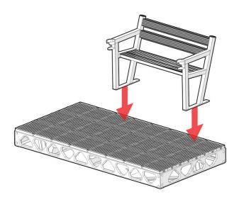
Place bench on dock to your desired location. Line up holes on bottom bracket to the holes on the decking.
