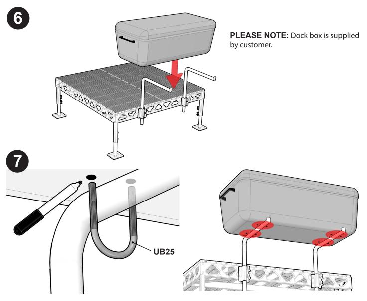
Approximate the position for all 4 U-Bolts(UB25) and mark holes for drilling.
