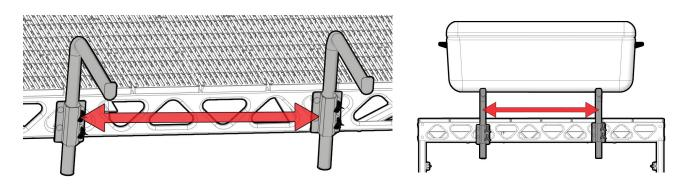
Spread brackets the appropriate amounts of spaces apart to accommodate the bottom of your dock box.
