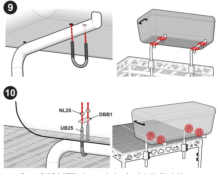
Connect all 4 U-Bolts(UB25) and necessary hardware from the inside of the dock box.
