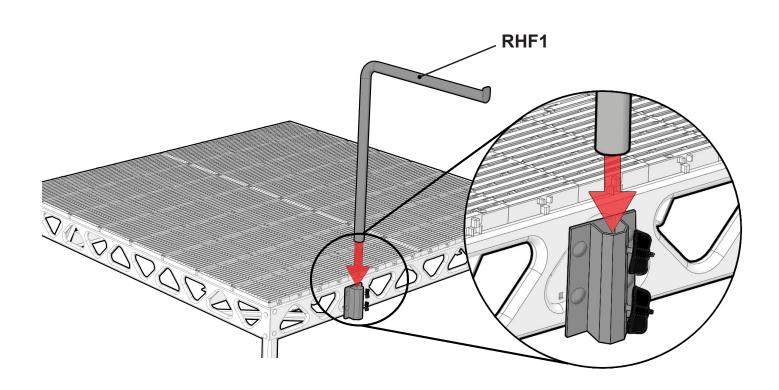
The height of your dock box may be adjusted by sliding the rack frame(RHF1) up or down to the height you require and tightening the adjustment knobs(AK1).
