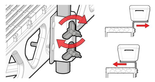
After you have adjusted the height of the rack frame(RHF1) to the desired height for your dock box tighten the adjustment knobs(AK1).
