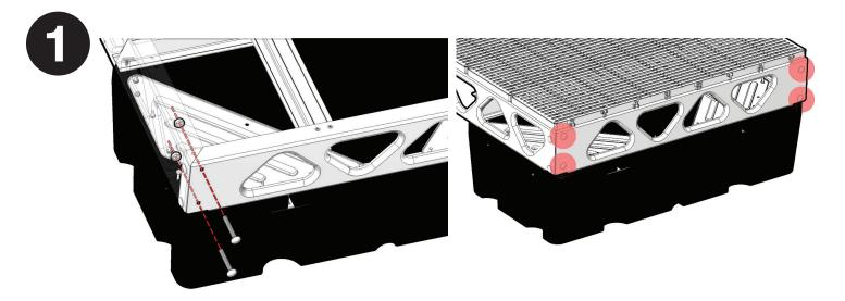
Remove existing carriage bolts to accommodate the mounting bracket (**SDMB2**). Repeat this step for both side of the dock.
