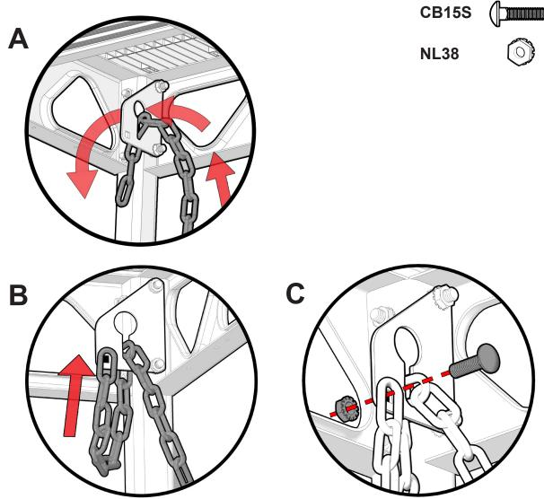
Feed the chain through the chain retainer keeping the chain link tight.
