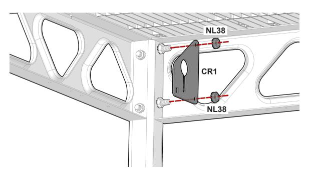
Place chain retainer(CR1) plate over top of existing bolts on corner legs. Fasten with nuts (NL38). Follow Step 1 for any other chain retainers to be added to your dock system.
