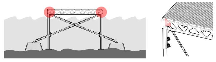
Chain retainers are used to connect anchor chains to a standing dock. See the images above to see locations for placement. Please view anchoring instructions for any further information on anchor installation and placement.
