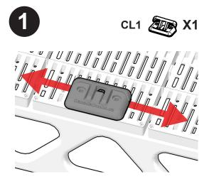
Position cleat ensuring that the holes of the cleat align with the slots on the decking. The flip-up portion of cleat should be opposite to the edge of dock.
