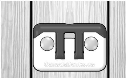
Position cleat in desired location on wood decking. Ensure flip up portion is opposite the edge of deck.
