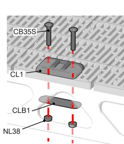
Position cleat ensuring that the holes of the cleat align with the slots on the decking. The flip-up portion of cleat should be opposite to the edge of dock.
