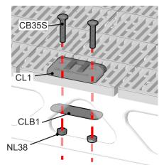
Insert carriage bolts and backing plate. Connect lock nuts as shown. Keep assembly loose until end of step 3.
