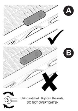
Ensure the backing plate of the cleat is placed over the lip of the truss (See image A). Do not position the backing plate on a bare section of decking (See image B). When the cleat has been positioned tighten the nuts to hold the cleat in place.
