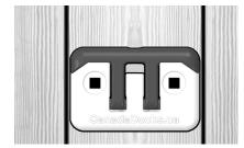
Drill holes and secure with appropriate fasteners.
