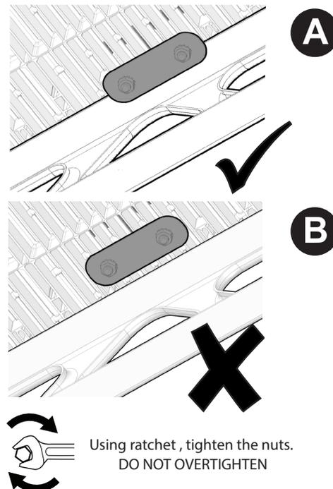
Ensure the backing plate of the cleat is placed over the lip of the truss (See image A). Do not position the backing plate on a bare section of decking (See image B). When the cleat has been positioned tighten the nuts to hold the cleat in place.
