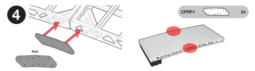
**PLEASE NOTE:** The arch on Connector (**CPRP1**) should be facing upwards. The two ramps will settle after the initial use to create a straight platform.
