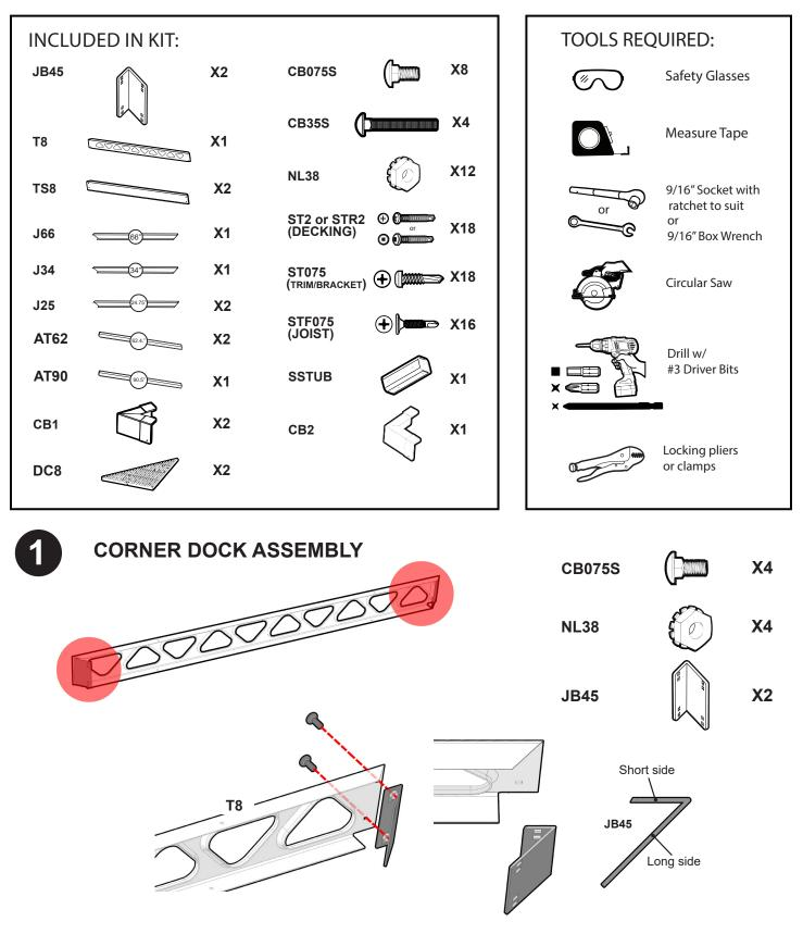
Ensure the short side of the bracket (JB45) faces the truss (T8).
