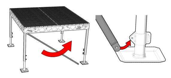
With the brace connected at one end place the opposite end between the two slots located on the edge of the jaw assembly (See image above).
