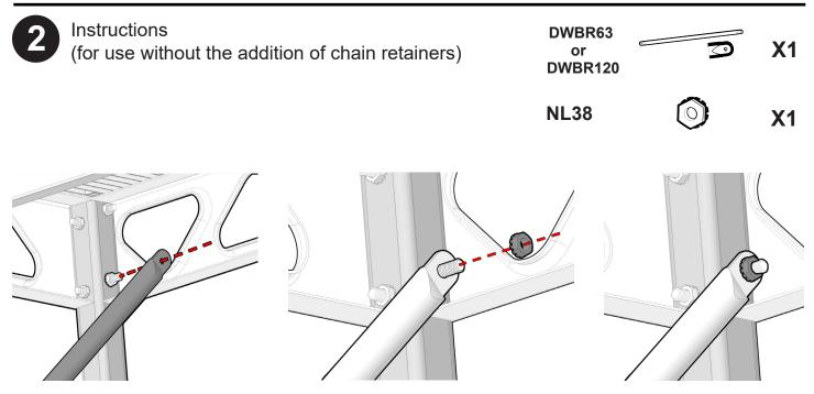
Install brace to the inside of the dock leg (See image above). Place overtop of the existing locknut and fasten with a new lock nut (NL38). Follow **Step 2** for any additional braces.
