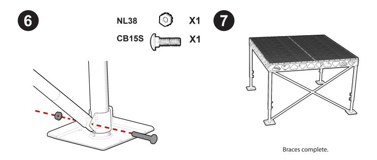
Fasten the brace end with a carriage bolt(CB15S) and locknut(NL38). Tighten both ends of the brace. Repeat Steps from the beginning of the instruction to connect the second brace to the dock.
