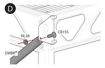
Fasten brace with carriage bolt and locknut. **PLEASE NOTE:** Only hand tighten the nuts so the brace moves freely for **Step 5**.
