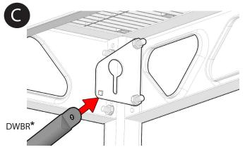
Place top hole of brace onto the hole of the chain retainer (See image above).
