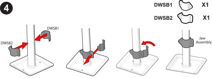
Fasten both jaws (DWSB1 & DWSB2) together on the leg. Repeat **Step 3** for other legs that any installed braces will be connected to.
