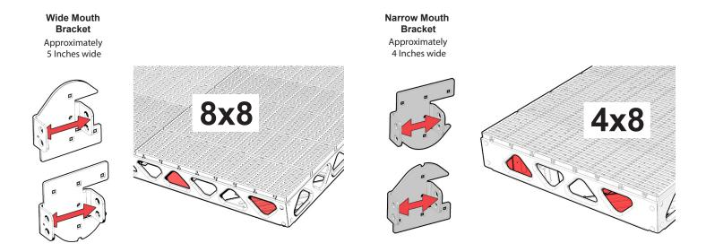
The wide mouth brackets will be installed on the 8x8 docks and the narrow brackets will be installed on the 4x8 docks.
