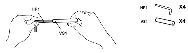
An optional sleeve(VS1) has been included with your kit to dampen any movement and sound that may arise from hinge use. Slide the vinyl sleeve unto the end of the pin(HP1).
