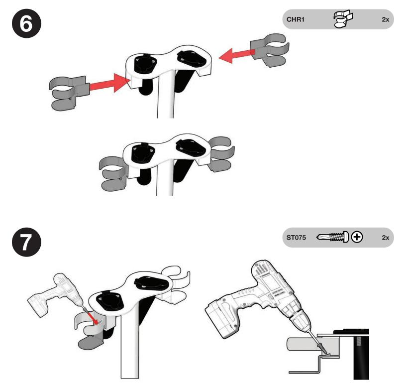
Add screw to fasten the cup holder. Repeat for cupholder on the opposite side of the fishing rod holder.
