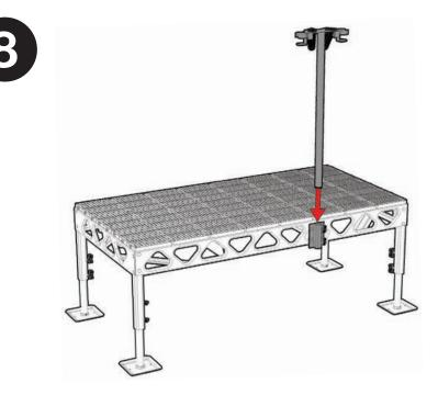
Adjust the stand to be at a comfortable height for holding your fishing rod.
