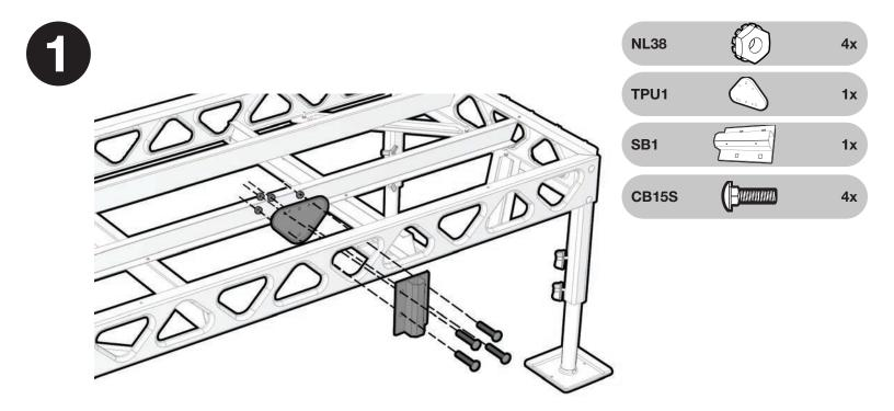
Install the bracket for the fishing rod holder in your desired location. Ensure the bracket does not obstruct any out accessories installed on your dock. Assemble as shown above.
