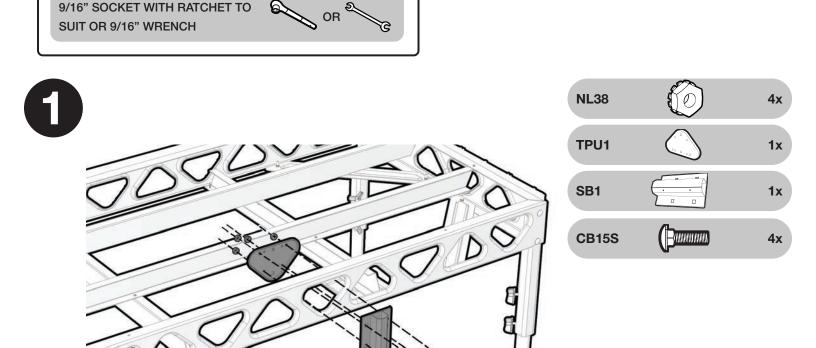
Install the bracket for the fishing rod holder in your desired location. Ensure the bracket does not obstruct any out accessories installed on your dock. Assemble as shown above.
