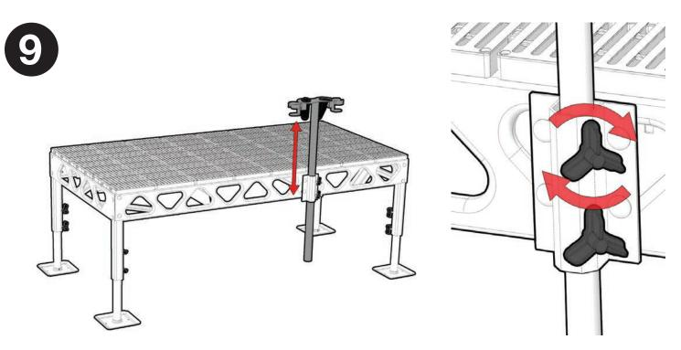
Once you have determined the rod height tighten both adjustment knobs.
