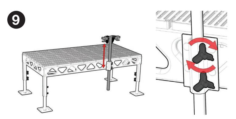
Once you have determined the rod height tighten both adjustment knobs.
