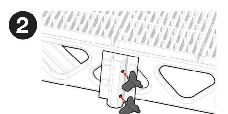
Connect the adjustment knobs (**AK1**) on the side of the bracket (**SB1**). Keep knobs loose to allow the fishing rod holder to slide into the bracket.
