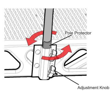
Setup your flag and flag pole according to the manufacturers instructions. Slide and place the base of the flag pole into the open hole at the top of the bracket. Turn and position the flag pole so that the pole protector is directly aligned with the adjustment knobs.
