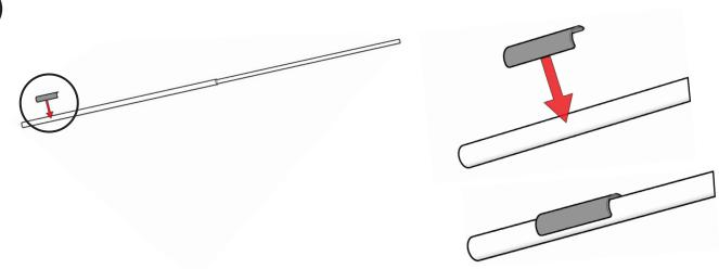
Apply the pole protector onto the flag pole. This component will be used to protect the pole when it is tightened and will need to be positioned near the base of the pole so it will be covered by the mounting bracket.
