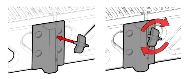
Insert adjustment knob (AK1) and turn handle clockwise to secure to the flag pole holder (See above). Turn the knob only enough times so that it is secure on the flag pole holder. Follow this procedure for bottom knob.
