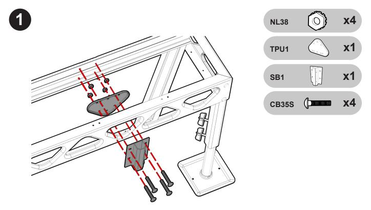
Find an appropriate triangle slot in your dock which will accommodate the flag holder (FH1). Ensure the slot will not be in the way or interfere with other dock accessories. Assemble flag pole on dock (As shown above).
