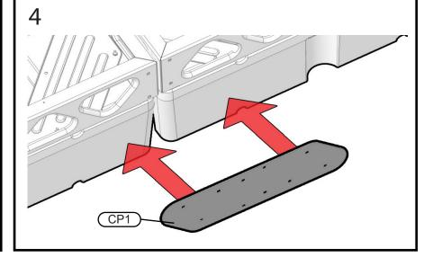
**PLEASE NOTE:** Some details such as decking has been removed to better illustrate assembly. TIP: Adjust dock height to align holes. Pry bar may help. Mallet or soft faced hammer may be needed to encourage bolts into place.
