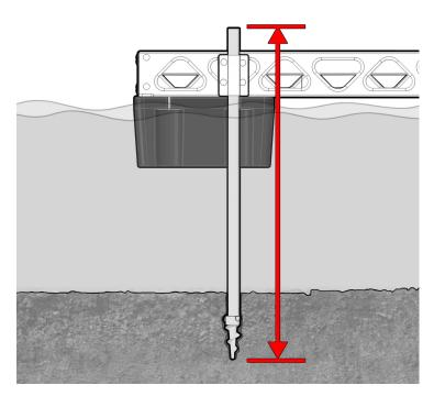
Length of stabilizer post should be determined by the depth needed for your dock's water level.
