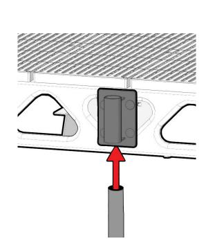
Slide and place the end of the EMT tubing into the stabilizer bracket until it reaches through the top of the bracket.
