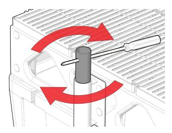
Using a long screwdriver or rod insert to twist the auger into the lakebed until it is secure.
