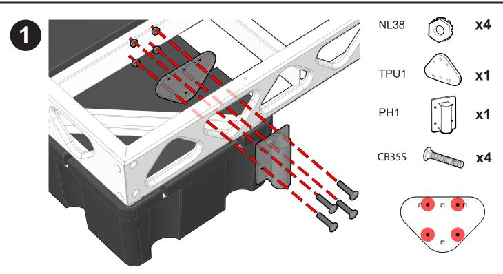
Find an appropriate triangle slot in your dock which will accomodate the bracket (PH1). Ensure the slot will not be in the way or interfere with other dock accessories. Assemble stabilizer bracket on dock (As shown above).
