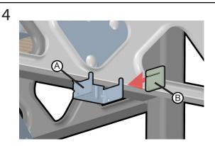
Slide Locking Key (B) onto the truss edge next to the Hanger Bracket(A).
