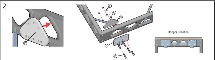
Take triangle Backing Plate (D) and place on the inside of the last triangle cut out of the 4' Truss. Connect Hanger Bracket (A) to Backing Plate(D) using 3/8" Carriage Bolts (E), Hex Nuts (F) and LockWashers(G). Follow this same step to add a Hanger Bracket on the opposite end of the 4' Truss (see above).
