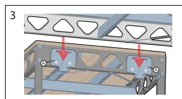
Place dock onto Hanger Brackets (A) to form a T-shaped configuration.
