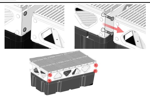
Using a socket/ratchet or box wrench, loosen carriage bolts on both dock or ramp that you will be attaching the hinge cover to (See image above for carriage bolt locations).
