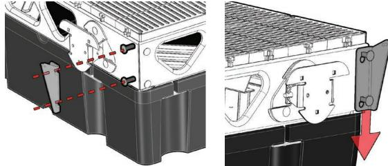
Repeat STEP 2, attach the right sided hinge cover bracket (HBR1) by loosening the carriage bolts and sliding the bracket (HBR1) down on the carriage bolts until they are seated in the narrow slots of the bracket.
