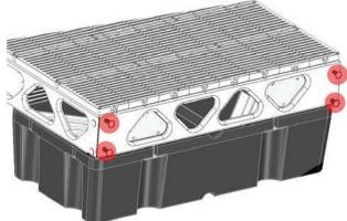
Using a socket or box wrench, loosen the carriage bolts on the dock section that you'll be attaching the hinge cover to (**see image above**).
