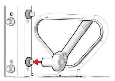
Retighten the carriage bolts on both brackets that were installed.
