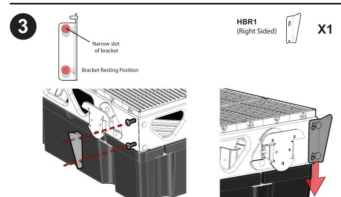
Attach the hinge cover bracket(HBR1) to the loosened carriage bolts at the end of the dock or ramp. Slide the hinge cover bracket(HBR1) down on the carriage bolts until they are seated in the narrow slots of the bracket.
