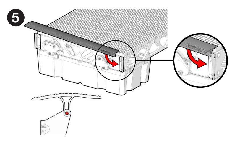
Position and slide the hinge cover onto the pin located at the top of the right sided bracket (**HBR1**).
