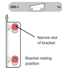
Attach the hinge cover bracket (HBL1) to the previously loosened carriage bolts on the left side of the dock or ramp. Slide the bracket (HBL1) down on the carriage bolts until they are seated in the narrow (square) slots of the
