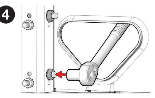
Re-tighten the carriage bolts on both brackets that were installed.
