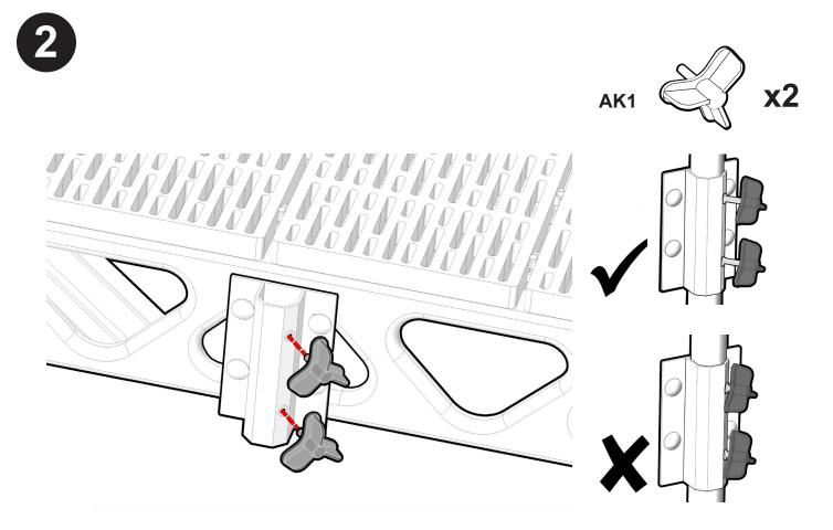
Connect the clamping knobs (AK1) to the side of the rack holder (RH1). Keep knobs loose to allow the rack/holder to slide into position.
