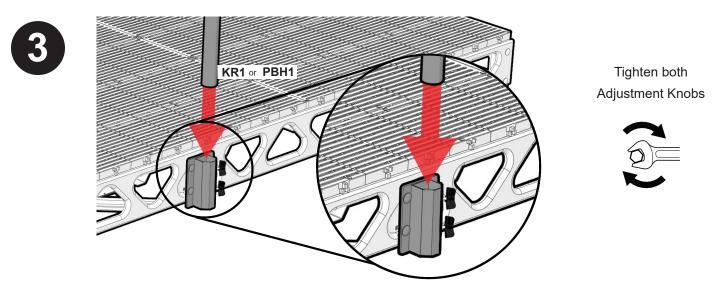
Adjust the height of rack/holder (KR1/PBH1) and tighten both adjustable knobs (AK1) by turning the handles clock-wise. Follow steps 1-3 for installing the second paddle rack/kayak rack and holder bracket.
