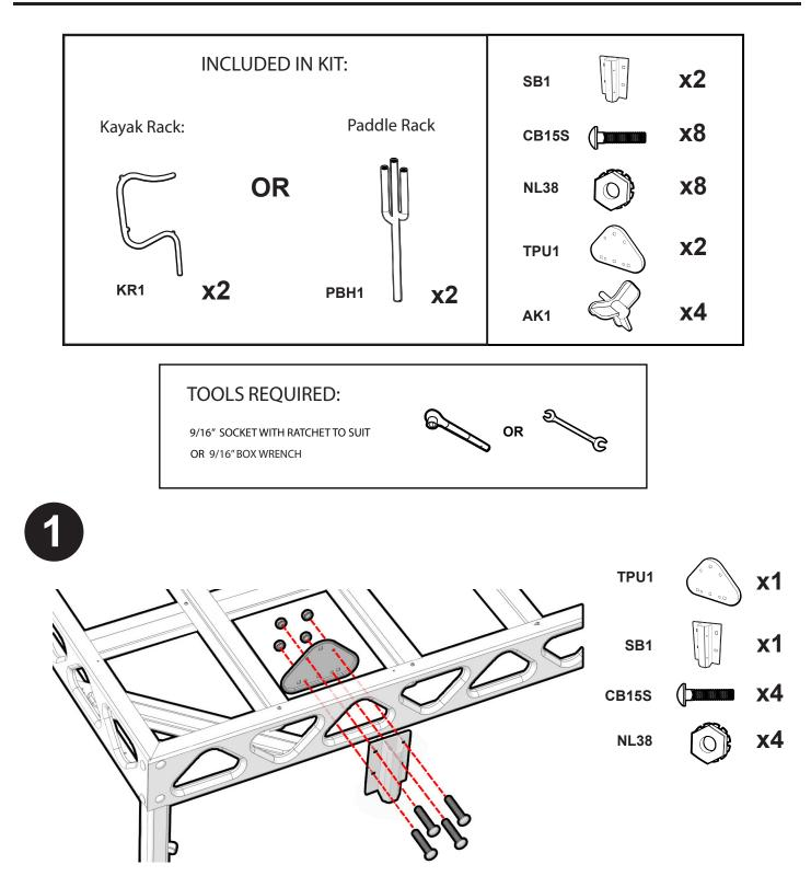
Connect the rack holder bracket (SB1) and triangle plate (TPU1) to the truss using carriage bolts (CB15S) and lock nuts (NL38). **PLEASE NOTE:** The decking has been removed from the image to better illustrate installation.
