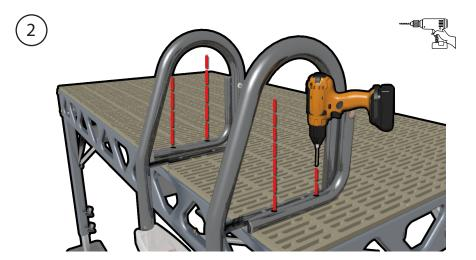
With the ladder frame flush against the dock use the L-Shaped Bracket holes as a guide to drill through the surface of the decking to accommodate the hardware for fastening the ladder to the dock. Drill holes on one side of the ladder before continuing the opposite side.
