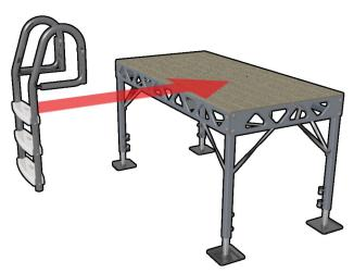
Place ladder assembly onto the dock. PLEASE NOTE: Ensure that the ladder is placed in an area that will not interfere with accessories connected to the dock. It is possible the ladder can interfere with accessories or other items placed on the dock when it is in the flipped up position.
