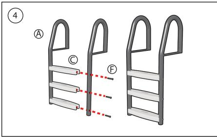
Connect the steps to the ladder using the Step Bolts (F) on the opposite side of the ladder.
