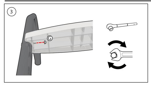
Apply a Lock Nut (G) hand tight to each Step Bolt (F) that connects the steps to the frame. After adding all Lock Nuts (G) to the frame, tighten each connection completely.
