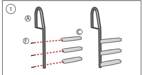
Connect the steps to the ladder using the Step Bolt (F).
