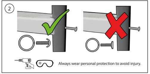
Ensure the curved head of Step Bolt (F) matches the profile of the ladder frame. (See above). If it does not than it is possible that the Lock Nut (G) will not fit on the end of the bolt. If you are finding it difficult placing the carriage bolt through the ladder frame holes simply drill through each hole with a 13/32" drill bit.
