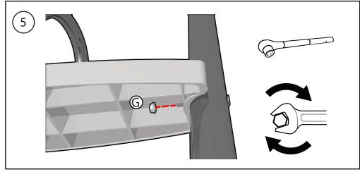
Apply a Lock Nut (G) hand tight to each Step Bolt (F) that connects the steps to the frame. After adding all Lock Nuts (G) to the frame, tighten each connection.
