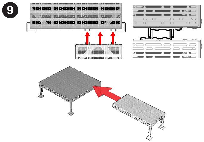
Once the brackets on both docks are assembled pull both docks close to each other. Place the docks so the edges of both docks are aligned with one another. Align the brackets on either side of the docks so they fit into each other (See images above). Ensure that the holes between both brackets line up with one another. Do the same for both hinge assemblies.
