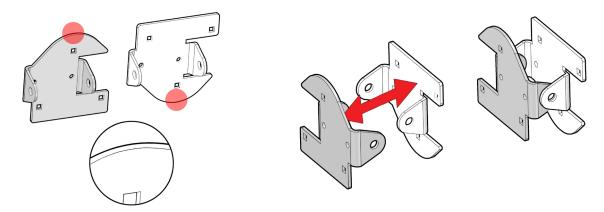
Two brackets will have no cookie cutter pattern on them. One bracket will have a narrow mouth that will fit into the wider bracket to create a hinge. These brackets will be paired together to make one hinge.
