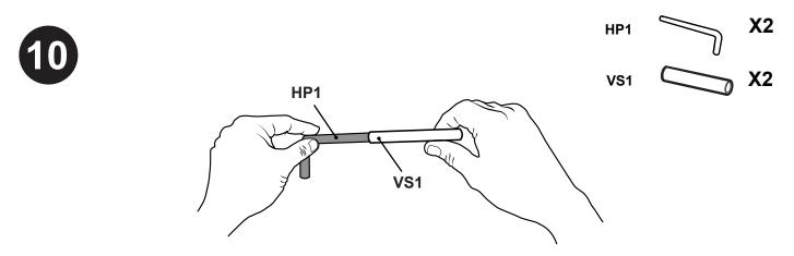
An optional sleeve(VS1) has been included with your kit to dampen any movement and sound that may arise from hinge use. Slide the vinyl sleeve unto the end of the pin(HP1).
