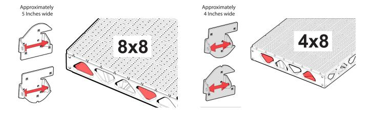
The wide mouth brackets will be installed on the 8x8 docks and the narrow brackets will be installed on the 4x8 docks.
