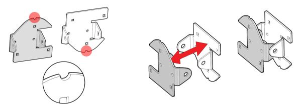
This kit contains four brackets. Two brackets will have a cookie cutter pattern on the top of the bracket.
