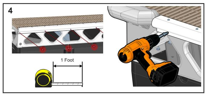
Place and drill your initial screw 1 inch from the end and then every foot along the P-Bumper. Putting a screw approximately an inch near both ends of the P-Bumper will help ensure the bumper does not rip off the dock.
