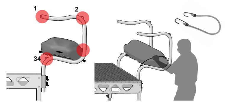
Bungie cables may be used to securely strap watercraft in place.
