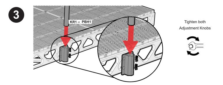
Adjust the height of rack/holder (KR1/PBH1) and tighten both adjustable knobs (AK1) by turning the handles clock-wise. Follow steps 1-3 for installing the second paddle rack/kayak rack and holder bracket.
