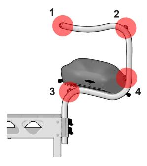
Each Kayak Rack frame has 4 hitch points for securing watercraft.
