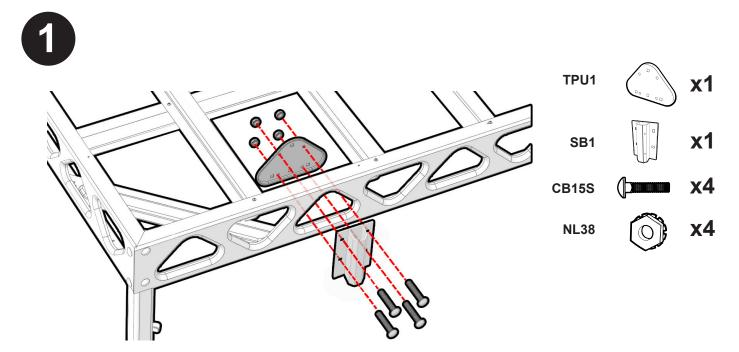
Connect the rack holder bracket (SB1) and triangle plate (TPU1) to the truss using carriage bolts (CB15S) and lock nuts (NL38). **PLEASE NOTE:** The decking has been removed from the image to better illustrate installation.
