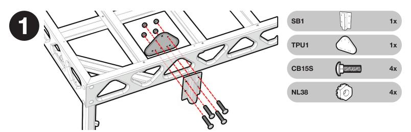
Connect the rack holder bracket (**SB1**) and triangle plate (**TPU1**) to the truss using carriage bolts (**CB15S**) and lock nut (**NL38**).
