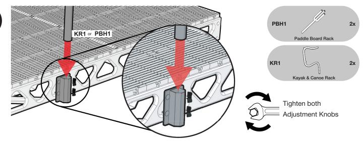
Adjust the height of the rack (**KR1** or **PBH1**) to the height you prefer and tighten both adjustment knobs (**AK1**) by turning the handles clockwise. Follow **STEPS 1-3** for installing the second paddle rack/kayak rack and bracket.
