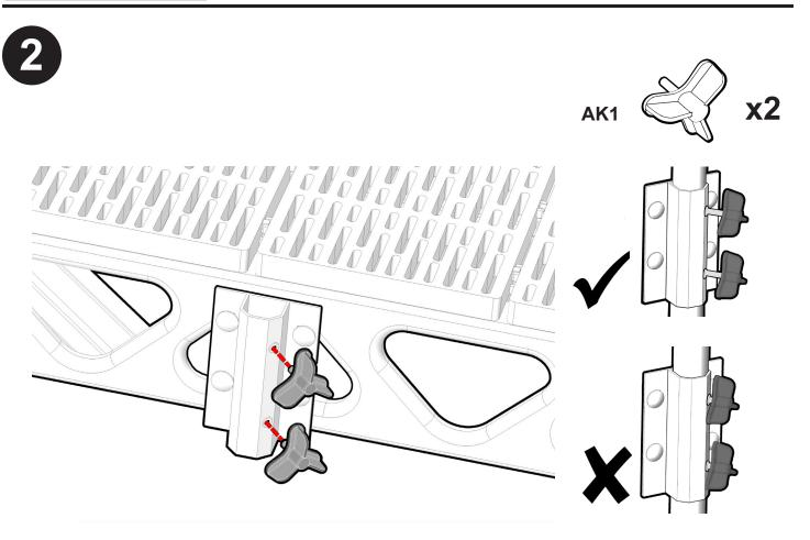
Connect the clamping knobs (AK1) to the side of the rack holder (RH1). Keep knobs loose to allow the rack/holder to slide into position.
