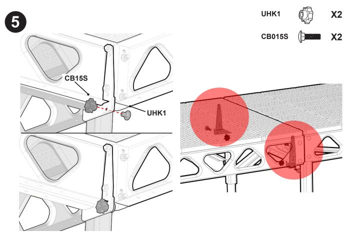
Align holes of both brackets and insert Bolt (CB15S). Fasten bolt with Knob (UHK1).
