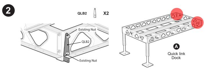
Remove the existing locknuts. Position the Joining Bracket (QLB2) on the bolts and fasten with existing nuts. Repeat Step 2 for the opposite side of the dock.
