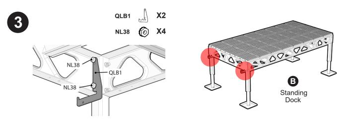
Position the "L" Shaped Bracket (QLB1) on top of current locknuts. Fasten the L-Bracket with Locknuts (NL38). Repeat Step 3 for opposite side of the dock.
