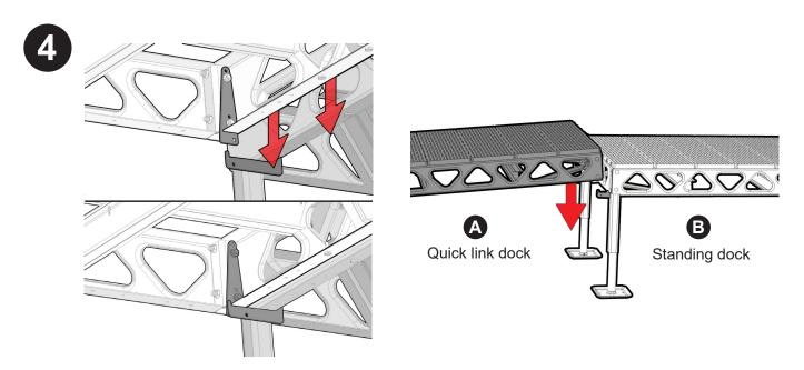
Decking can now be installed on your dock. After decking has been finished you may lower the quick link dock **A** onto the "L" Shaped Bracket (QLB1) of the existing standing dock. **B**
