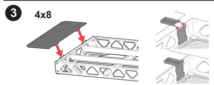
Slide the hinges of the assembled plate onto the hinges of the dock frame. (See image above).
