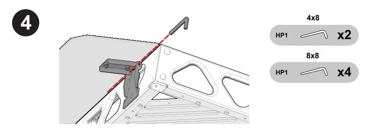
Slide the hinge pin (HP1) into the hinge from the outside of the dock. Add pins to all hinges on the truss. (See image above).
