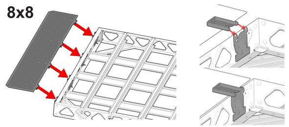
Slide the hinges of the assembled plate onto the hinges of the dock frame. (See image above).
