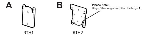
Each hinge for the transition plate consists of the following parts:
