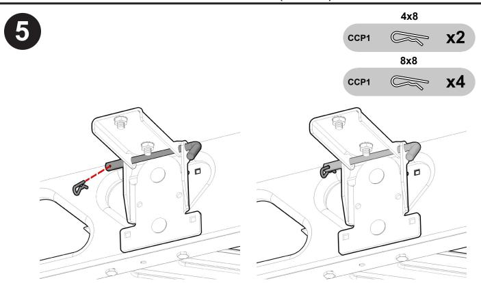
Slide the cotter pin (CCP1) into the hinge pin. Insert a cotter pin for all hinge pins. (See image above).
