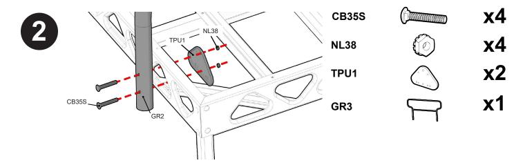
With one person holding the railing level place the **Triangle Backing Place(TPU1)** on the inside of the truss triangle cutout and fasten. Do this for both ends of the Hand Railing frame.
