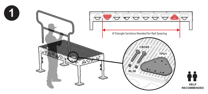
Find an area on your dock that will have 8 triangle sections between the railing. Organize and set all the hardware you will need (Items TPU1,CB35S,NL38) onto the decking near each point of fastening. Using the help of another person, hold the end of the railing level near the triangle cutout where it will be installed.
