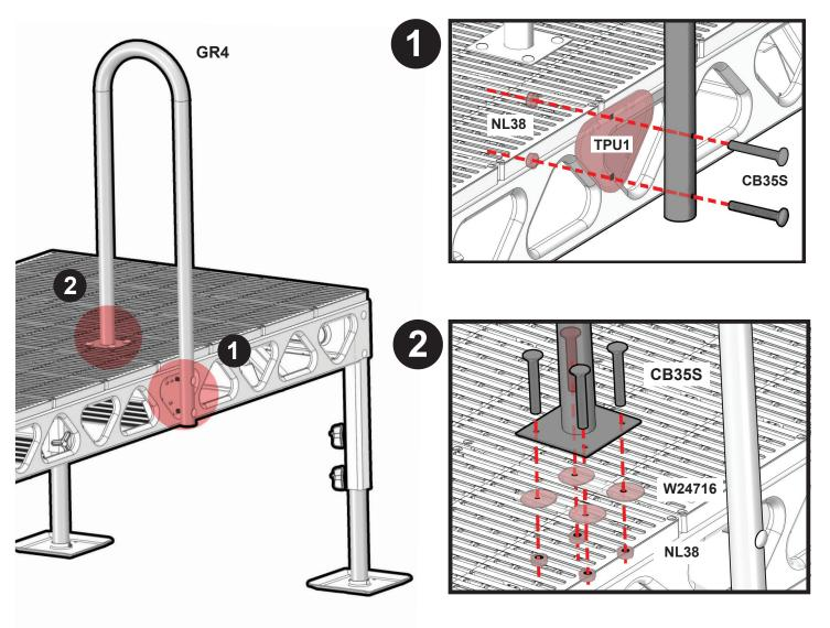
**NOTE:** You may configure the back plate upwards or downwards on the dock depending on where you wish to place the safety grab rail on the dock.
