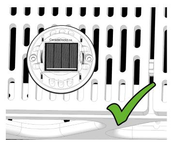
Place the solar light in a suitable location on the decking. Ensure the solar light is positioned so both screw holes are on top of a solid backing for fastening.
