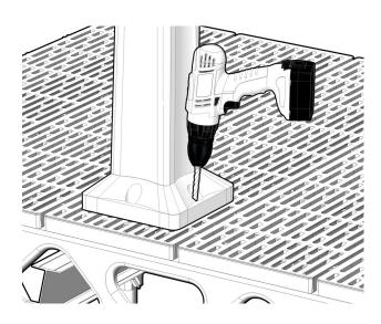
Depending on where you mount your solar post on the dock it may be necessary to drill some holes to accommodate the bolts that secure the post.
