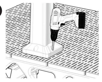
Depending on where you want your solar post on the dock it may be necessary to drill some holes to accomodate the bolts that sure the assembly.
