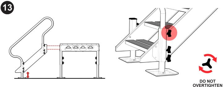
Adjust the legs so the base of the stairs sits approximately at the height as the dock. Keeping the stairs level to the dock will make it easier for installation. After the legs are set snug the adjustment knobs.
