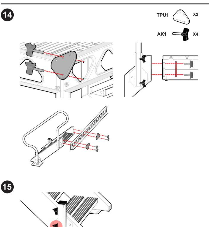
Adjust height of leg and tighten using the knobs shown.
