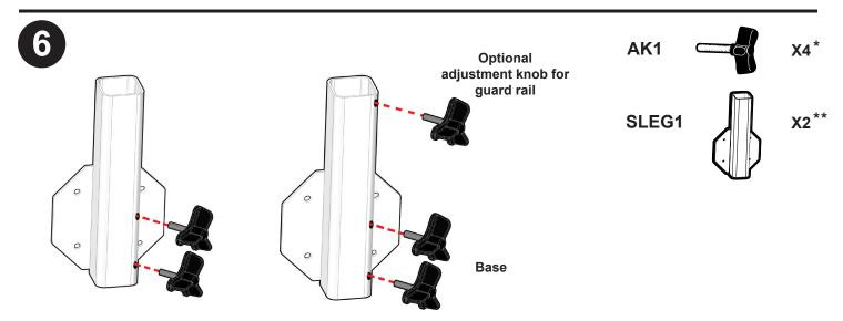
If you purchased stairs without the guard rail assemble two brackets with two adjustment knobs added to the base. If you purchased the optional guard rail assemble two brackets with 3 adjustment knobs and one bracket with 2 adjustment knobs added to the base.
