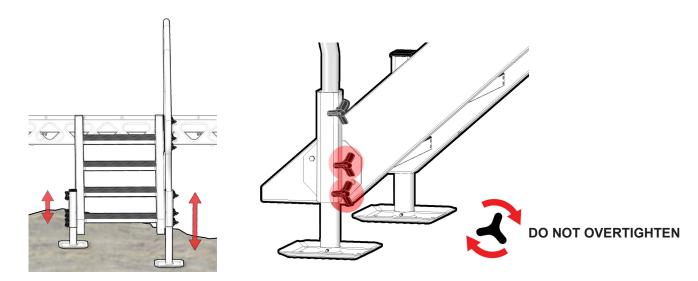
Readjust height of legs and tighten with the adjustment knobs shown. Adjust the legs according to your lake bed conditions.
