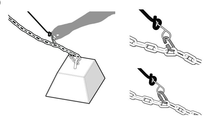
Attach the quick connector onto the bottom part of the chain that is easily accessible to you.
