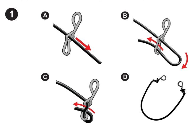
Assemble rubber cording and steel ends as shown above. Repeat Step 1 for both ends of the tension cord .
