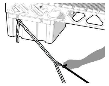
Pull the quick connector upwards towards the dock. When there is tension on the cord connect the quick connector onto the chain.
