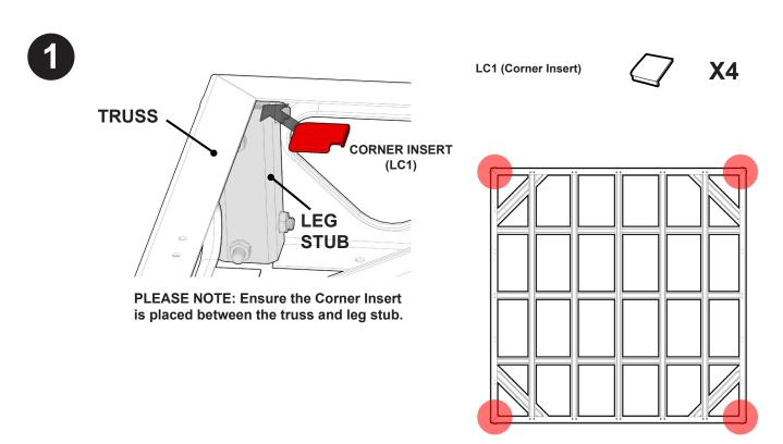
Install one Corner Insert (LC1) into each corner of the dock frame. Slide the Corner Insert completely between the lip of the truss frame and the corner leg stub (See sideview image above).
