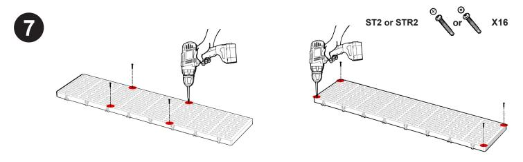
Recheck all spacing on panels. Ensure panels are aligned so they are flush with the dock frame. Fasten panels C & D starting from the middle, then the outside corner and finally the remaining corners.
