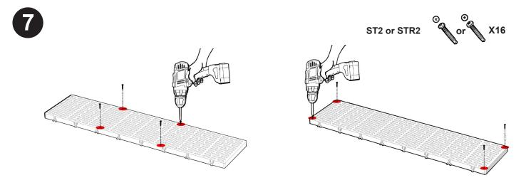
Recheck all spacing on panels. Ensure panel sets C & D are aligned so they are flush with the dock frame. Fasten each panel starting from the middle, then the outside corner and finally the remaining corners.
