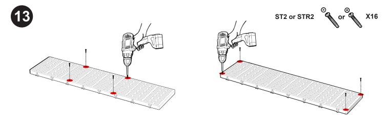
Recheck all spacing on panels. Ensure panel sets G & H are aligned so they are flush with the dock frame. Fasten each panel starting from the middle, then the outside corner and finally the remaining corners.
