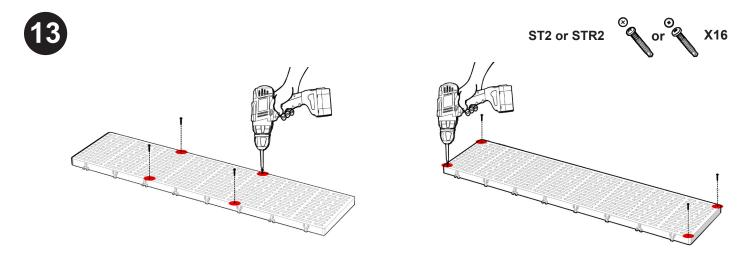
Ensure Thruflow TM (DK1x4) panels are aligned so they are flush with the dock frame. Fasten panels G & H starting from the middle, then the outside corner and finally the remaining corners.
