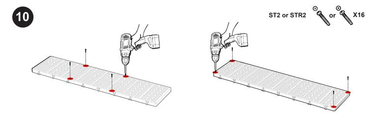
Recheck all spacing on panels. Ensure panels are aligned so they are flush with the dock frame. Fasten panels E & F starting from the middle, then the outside corner and finally the remaining corners.
