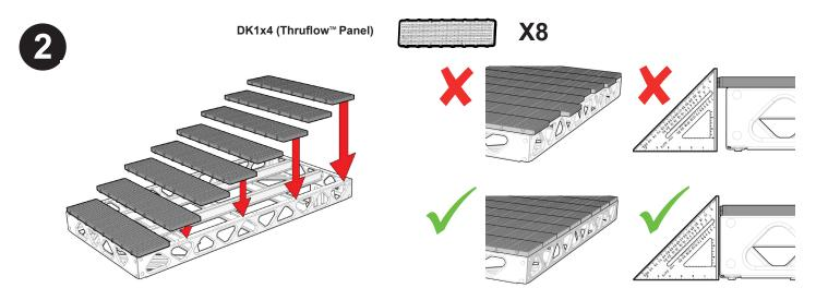
Place all 8 panels on the dock frame. Ensure decking is flush with dock frame.
