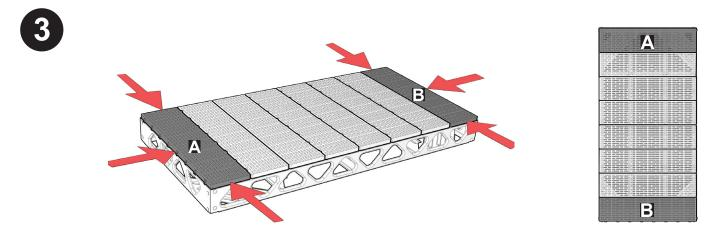
Align panels A & B so they are flush with the front and sides of the dock.
