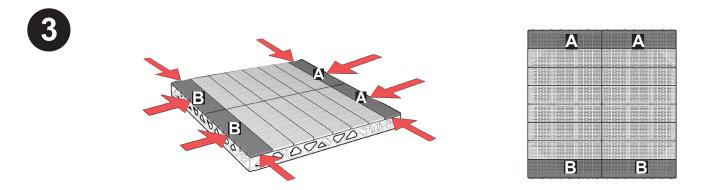
Align panel sets A & B so they are flush with the front and sides of the dock. Ensure that panels are aligned with the edges of the dock frame.
