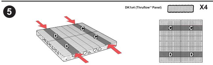
Place and align panel sets C & D so they are flush with the edges of the dock. Ensure that the panels are aligned with the edges of the dock frame.
