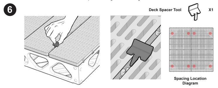
Use the Deck Spacer Tool (As shown above) to create a space evenly on both sides of panel sets C & D (See above diagram for locations).
