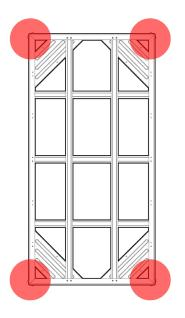
Install one Corner Insert (LC1) into each corner of the dock frame. Slide the Corner Insert (LC1) completely between the lip of the truss frame and the corner leg stub (See sideview image above).
