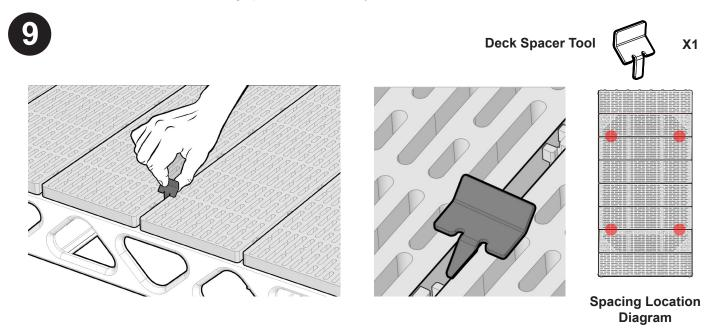
Use the Deck Spacer Tool (As shown above) to create a space evenly on both sides of each panel E & F.
