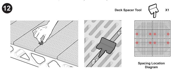
Use the Deck Spacer Tool (As shown above) to create a space evenly on both sides of panel sets G & H (See above diagram for locations).
