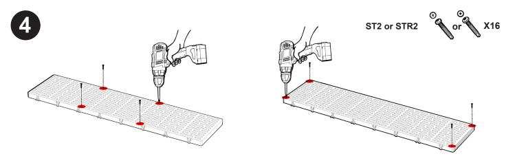
Ensure panels are aligned so they are flush with the dock frame. Fasten panels A & B starting from the middle, then the outside corner and finally the remaining corners.
