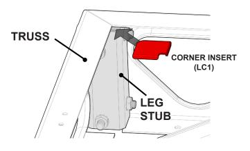
PLEASE NOTE: Ensure the Corner Insert is placed between the truss and leg stub.
