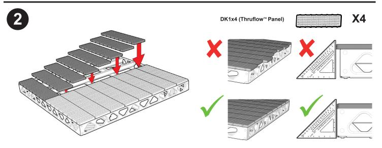
Place all 16 panels onto the dock frame. Ensure decking is flush with dock frame.
