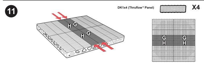
Place and align panel sets G & H so they are flush with the edges of the dock. Ensure that the panels are also aligned with the edges of the dock frame.
