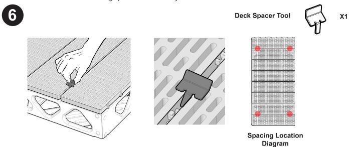
Use the Deck Spacer Tool (As shown above) to create a space evenly on both sides of each panel C & D.
