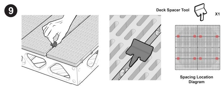
Use the Deck Spacer Tool (As shown above) to create a space evenly on both sides of panel sets E & F (See above diagram for locations).
