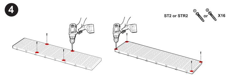
Ensure panel sets A & B are aligned so they are flush with the dock frame. Fasten each panel starting from the middle, then the outside corner and finally the remaining corners.
