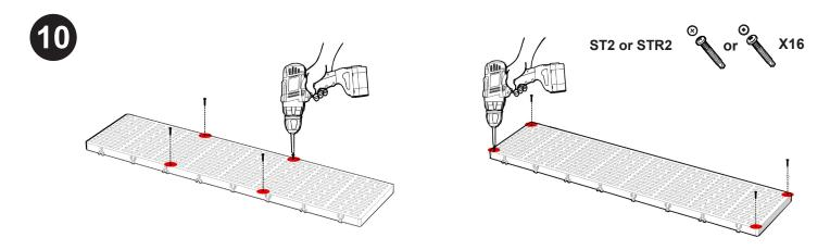
Recheck all spacing on panels. Ensure panel sets E & F are aligned so they are flush with the dock frame. Fasten each panel starting from the middle, then the outside corner and finally the remaining corners.
