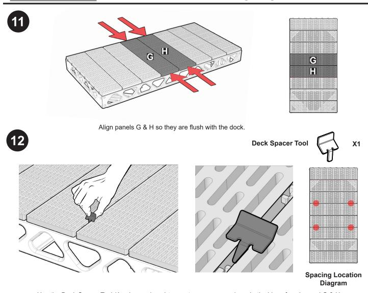
Use the Deck Spacer Tool (As shown above) to create a space evenly on both sides of each panel G & H.
