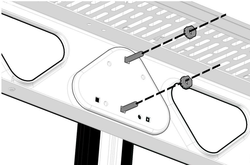
Using the lock nuts (**NL38**) fasten the assembly onto the dock as seen above.
