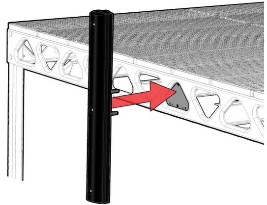
Feed the bolts on the bumper through the backing plate while holding it in place.
