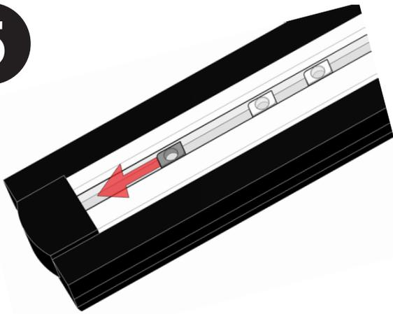
Only two square nuts are needed for fastening the vertical bumper to the dock. If your bumper has more than two nuts in the slot, you can hide the extras under the black sleeves at the end.
