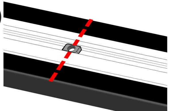
Place the square nut in the slider along the new mark.
