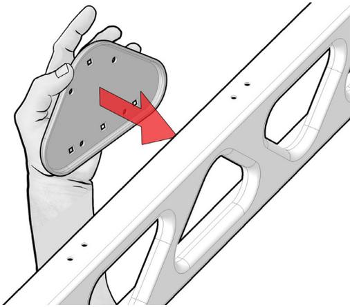
Find an appropriate location to mount the vertical bumper and place the triangle plate on the back of the truss.
