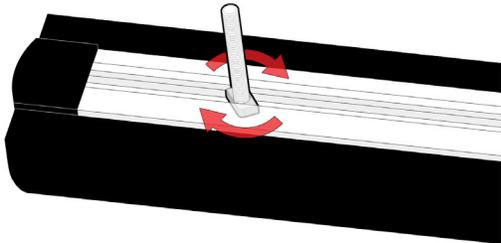
Twist the square nut inside the aluminum channel of the bumper until it locks to ensure it will not fall out. Hold your finger on the nut to prevent it from becoming misaligned. Tighten the rod.
