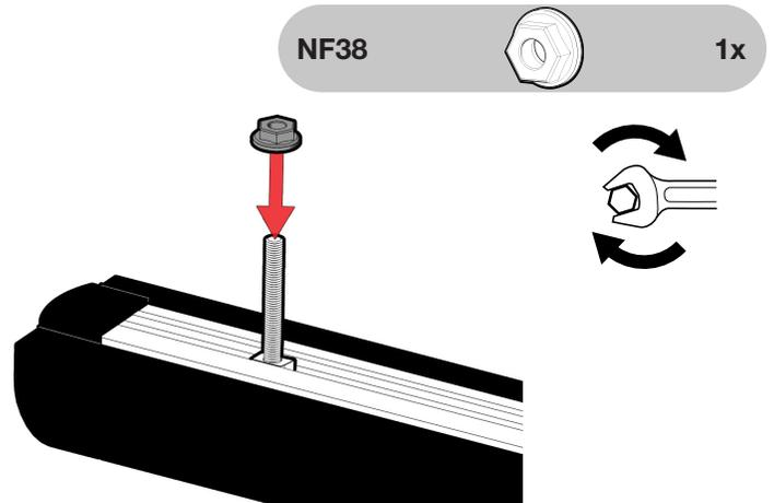
Fasten the flange nut (**NF38**) onto the rod. Hold the square nut to ensure it stays in play while tightening the assembly.
