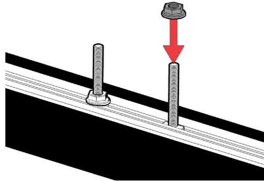
Fasten the flange nut (**NF38**) onto the rod. Keep loose so you may slide the bolt along the channel for the next step.
