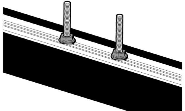
Tighten the flange nuts in place.
