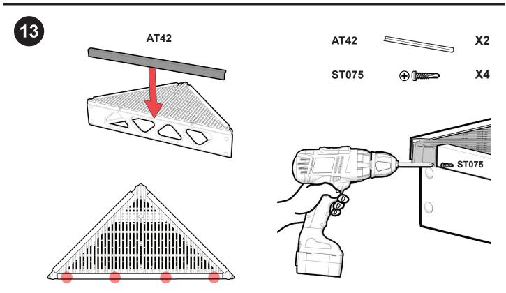
Fasten aluminum trim (AT42) on the truss frame with four screws (CB075S) through each piece of trim into the truss.
