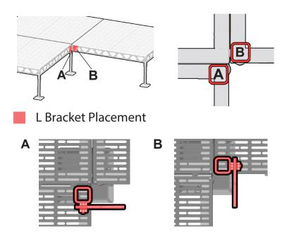
L-Bracket(QLB1) may be positioned on either Leg 1 or 2 as shown.
