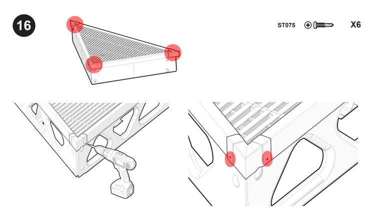
Fasten each bracket with two screws(ST075) in the locations shown Step 26.
