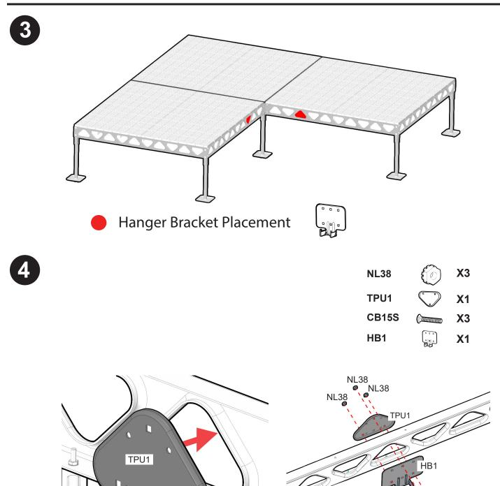
Place and install both hanger brackets (HB1) on the truss locations (see image in Step 3) on either side of the corner dock. **PLEASE NOTE:** The above image has hidden some deck elements such as decking to better illustrate the hanger bracket assembly.
