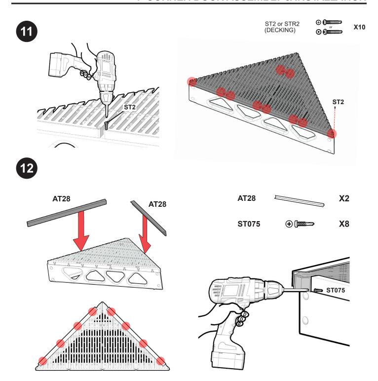
Fasten aluminum trim (AT28) around the two sides of the truss frame with four screws (ST075) through each piece of trim into the truss.
