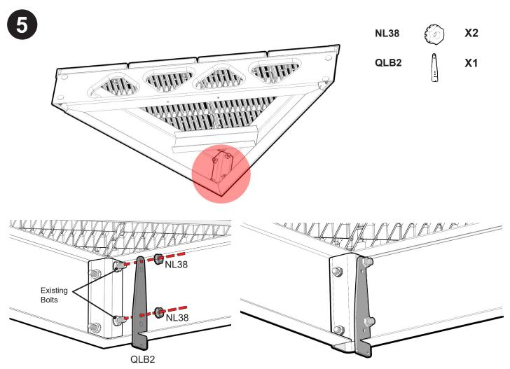
Fasten joining bracket (QLB2) to the corner dock in a position that will be parallel and on the same side as the L-Bracket from Step 2.
