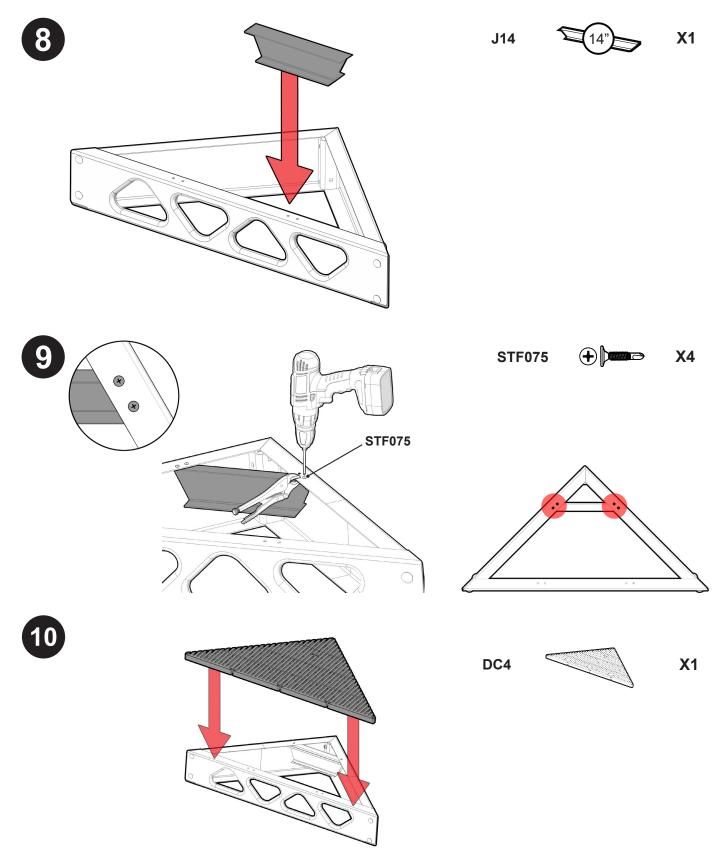
Clamp a sheet of ThruFlow™ decking (DC4) to the truss frame aligning the sheet with the triangle cut truss frame. The sheet, after aligned and centered, should cover the top of the truss frame (See above).
