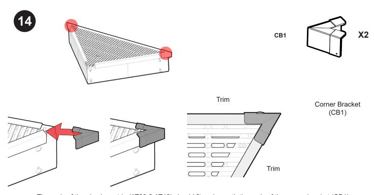
The ends of the aluminum trim(AT28 & AT42) should fit underneath the ends of the corner bracket (CB1).
