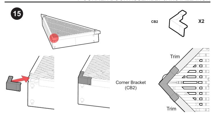
The ends of the aluminum trim(AT28) should fit underneath the ends of the corner bracket (CB2).
