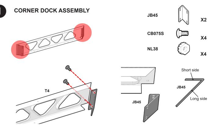
Ensure the short side of the bracket (JB45) faces the truss (T4). Follow Step 1 for the opposite end of the truss(T4).
